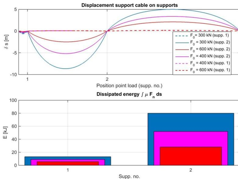
Fig. 3: Ideal gliding support cable on the towers for different cable tensions  $F_0$  at fixed temperature  $T_{curr} = 25 \text{ }^\circ\text{C}$ . A negative value for  $\delta_s$  means that the cable moves to the left (valley side). The data can help to estimate the possibility to bring the cable outside the support range for inspection using a sufficient point load. The lower part shows the heat production due to friction resistance during the ride, where the
