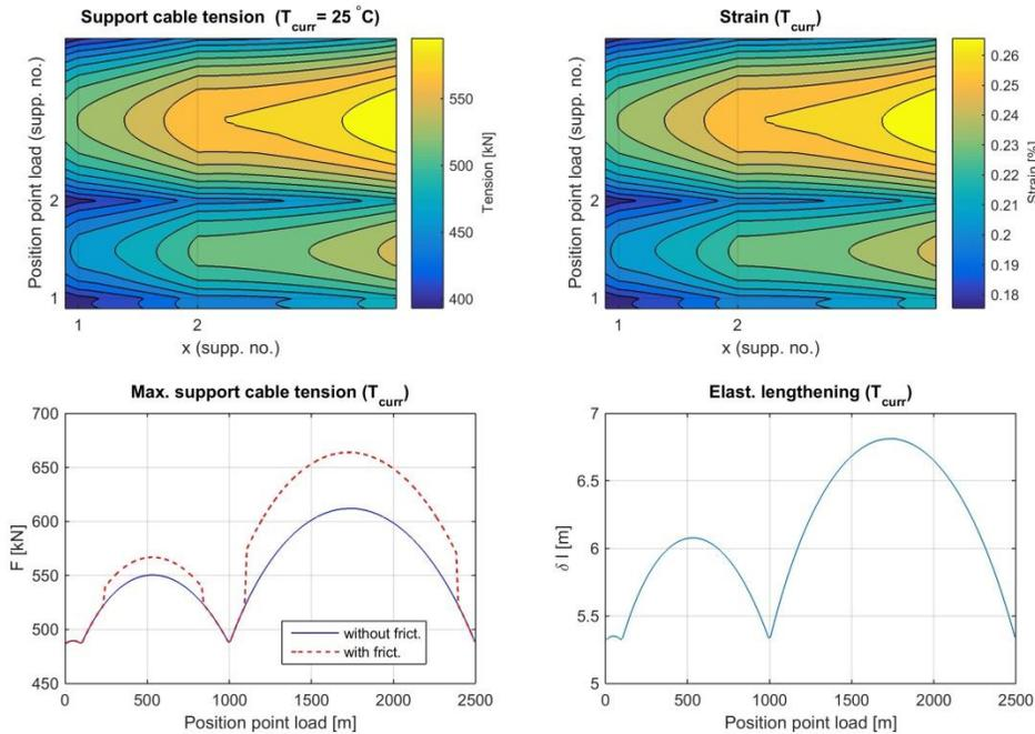
Fig. 2: Data for the support cable: cable tension as a function of  $x$  (horizontal) and point load position  $x_z$  (vertical), where no friction resistance on supports is assumed (left upper panel). The corresponding strain (right upper panel). The lower figures show the maximum value of the cable tension without and with friction resistance and the elastic lengthening of the cable computed in zeroth order, respectively.
